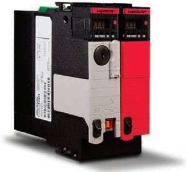
Once the project is tested and ready for final validation, you set the Safety Task to a SIL 3, PL<sub>e</sub> integrity level, which is then enforced by the GuardLogix controller. When Safety Memory is locked and protected, the safety logic can't be modified and all safety functions operate with SIL 3, PL<sub>e</sub> integrity. On the standard side of the GuardLogix controller, all functions operate like a standard Logix controller.
